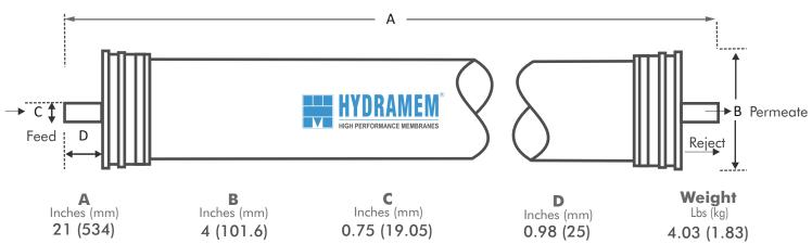
All Membrane Elements are supplied with a brine seal, interconnector and O rings
