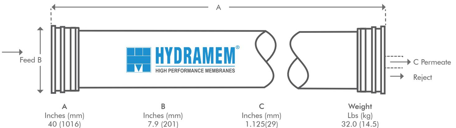
All Membrane Elements are supplied with a brine seal, interconnector and O rings
