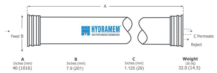
All Membrane Elements are supplied with a brine seal, interconnector and O rings
